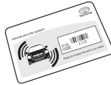
This code consists of four digits and allows you to activate / deactivate the alarm system manually (emergency override). Please refer to the "emergency override" section for the procedure to use this code.
