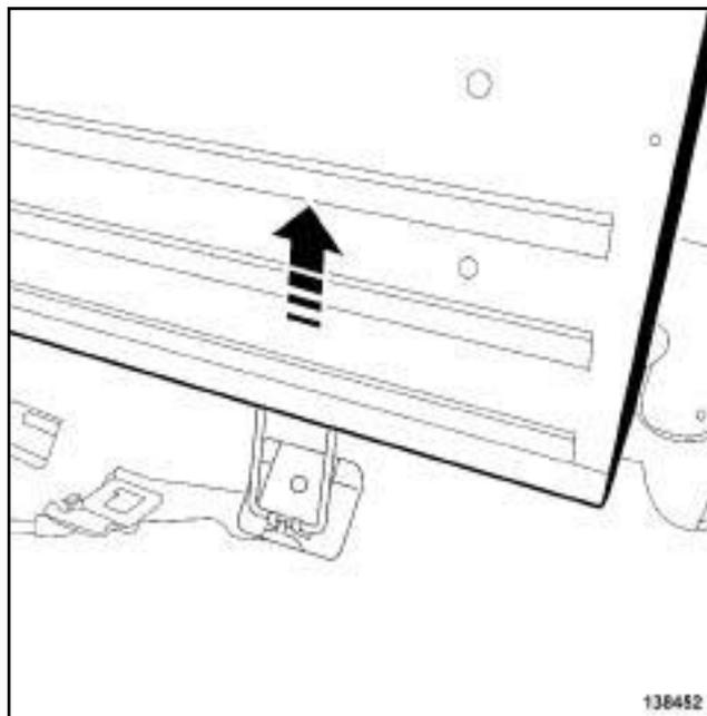
❑ Unclip the load stop floor at the retaining hooks.
