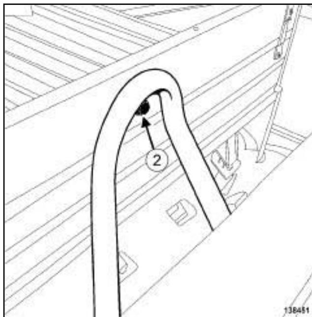
❑ Remove the bolt of the load stop bracket (2) .
