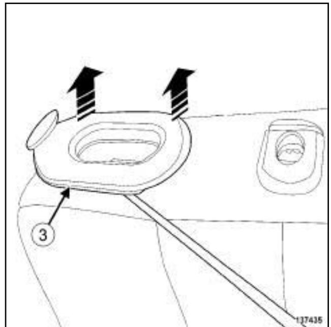
❑ Remove the bench seat lock trims (3) in order to tilt the seatback.
